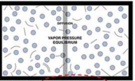
Equilibrium Conditions: After several hours or days, the higher concentration of water vapor polecules continues diffusing until a vapor pressure equilibrium is reached across both chambers.
