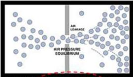
Equilibrium Conditions: After several seconds, the air/vapor mixture leaks from the left chamber into the right chamber ontil air pressure equilibrium is reached across both chambers.
