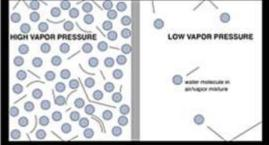
Initial Conditions: The higher temperature and water vapor content in the left chamber causes a vapor pressure gradient toward the right and drives the water vapor molecules through the vapour retarder.
