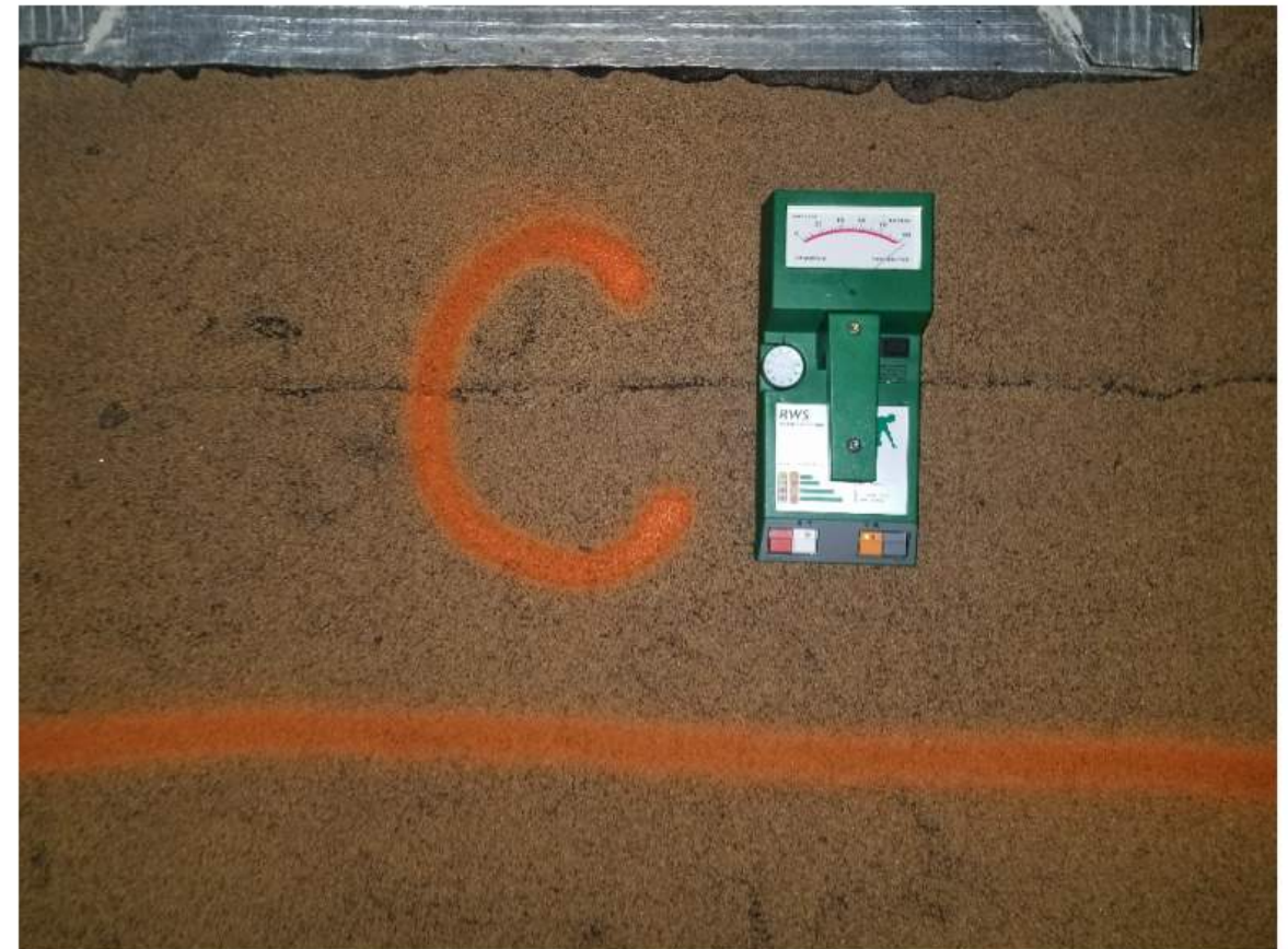
Image Set 3: Infrared image (left) displaying a thermal anomaly indicative of moisture infiltration surrounding the exhaust vent (Spot C). Non-invasive moisture readings at this location were elevated. The right image is a digital that displays the elevated moisture reading in the center of Spot C.
