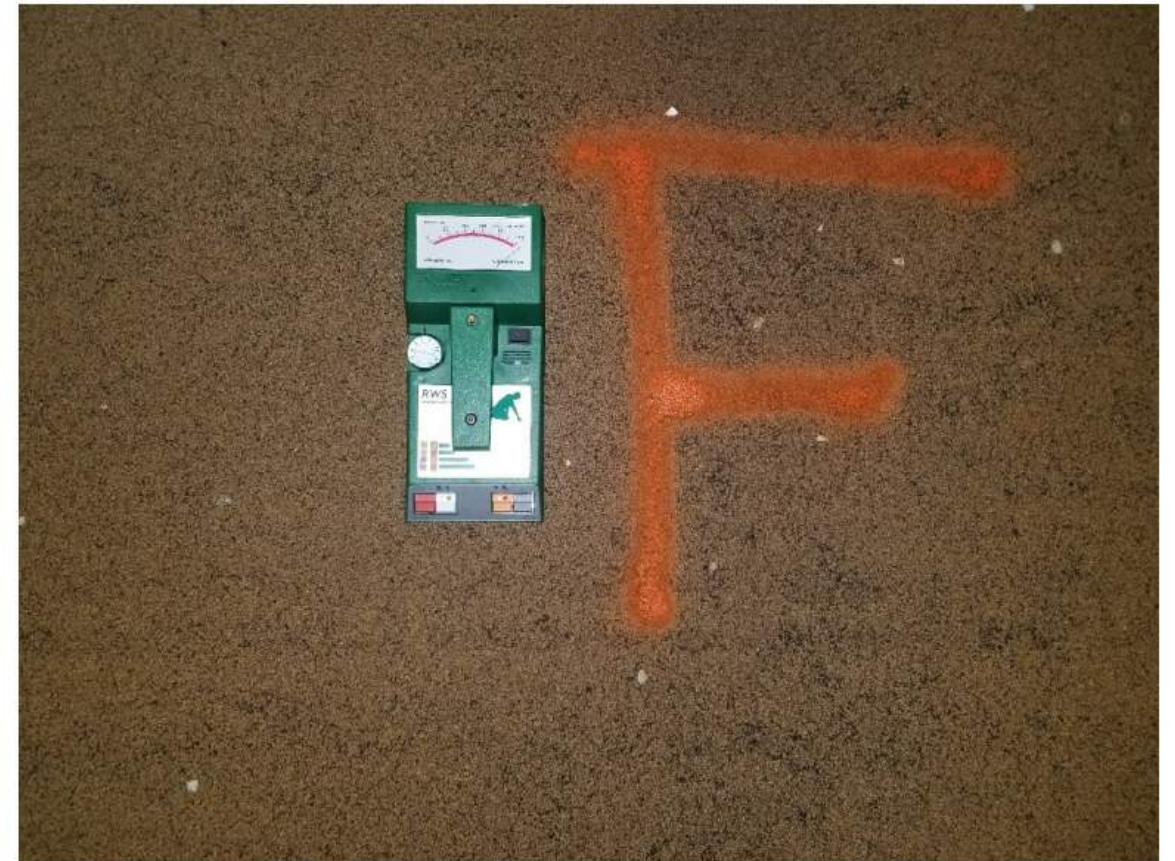
Image Set 4: Infrared image (left) displaying a large thermal anomaly extending down-slope (Spot F). Another anomaly can also be viewed in this image to the right of the exhaust vent (Spot E) The right image is a digital that displays the elevated moisture reading in the center of Spot F.
