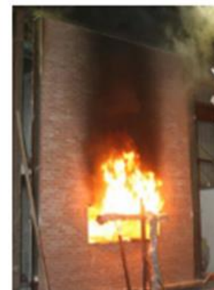
Reduced-scale Fire Test UBC 26-9 / NFPA 285
