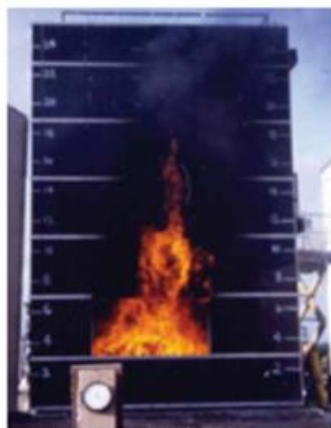
Full-scale Fire Test UBC 17-6 / UBC 26-4
