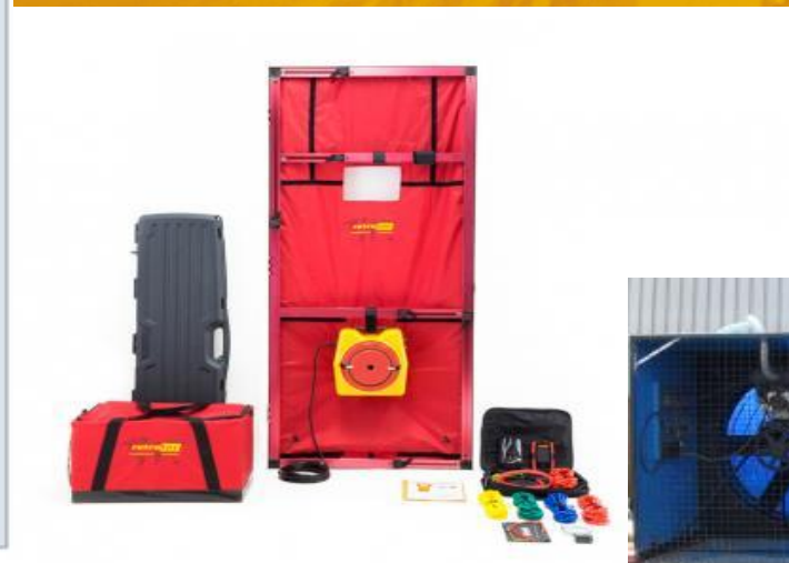
Standard Pressurization Kit and gauges used by Building Science Engineer Partner
