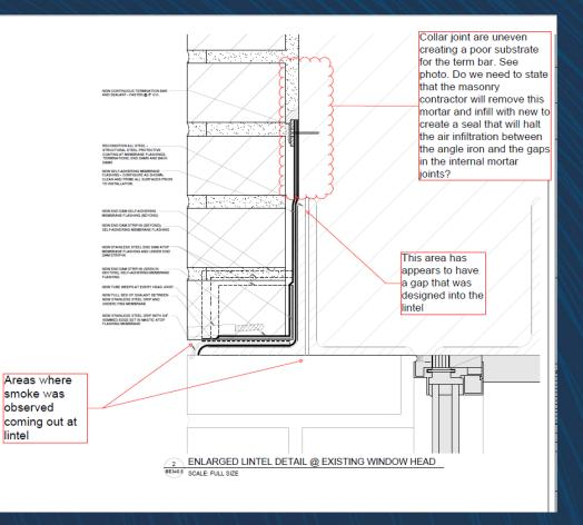
Windows not being sealed where frame meets wall. Seal the lintel from the inside during construct.
