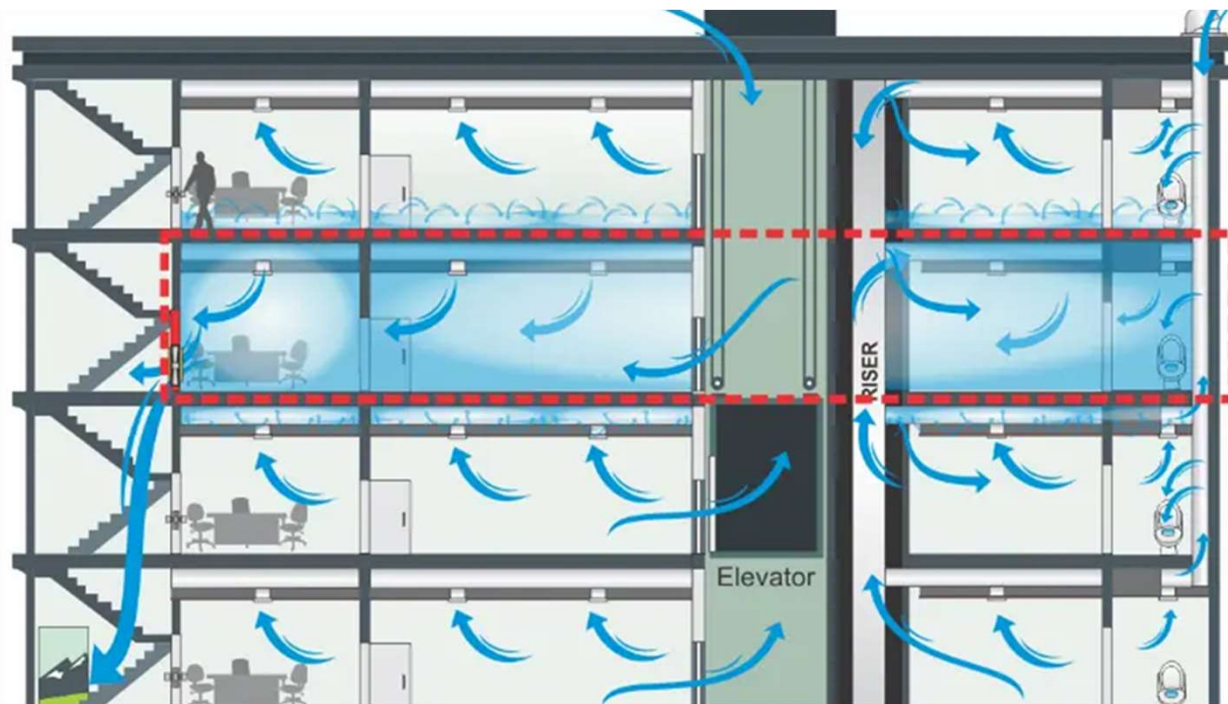
Floors (alone) Airtightness Test
